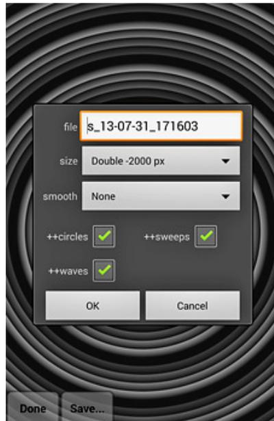
The important thing to note is that you can alter the size and quality of the saved image. Picture sizes vary from 100 pixels up to 1000/2000/4000, (the upper limit depending on the amount of internal memory in the Android device). In SourcesLite the image is restricted to screen size or 750 pixels, whichever is smaller.
